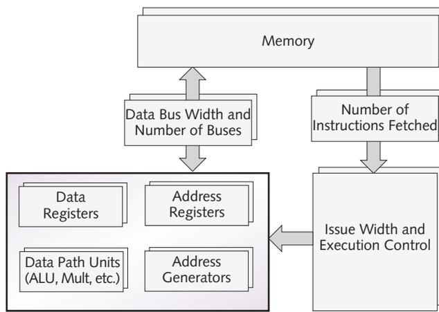
**Figure 4.** According to the StarCore partners, scalable features of the StarCore 400 architecture include data bandwidth, instruction issue width, function units, address generators, and registers.
