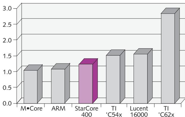
**Figure 3.** StarCore's benchmark results showing relative memory usage of the StarCore 400 architecture on compiled C and C++ code. According to Lucent and Motorola, these results are based on a subset of DSP, control, and encryption benchmarks drawn from Motorola's own "PowerStone" benchmarks.
