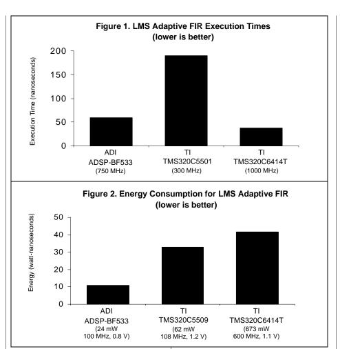
TMS320C5501 are both dual-MAC DSPs, only the ADSP-BF533 uses its dual-MAC capability on this benchmark. In the TMS320C5501, the two MAC units share an input-a restriction not imposed by most architectures. The TMS320C5501 is therefore limited to single-MAC operation on the filtering section of this benchmark. In contrast, the ADSP-BF533 is uses both of its MAC units on this benchmark. As a result, the ADSP-BF53xx is signifiefficient cantly more than the TMS320C5501 on this benchmark.
