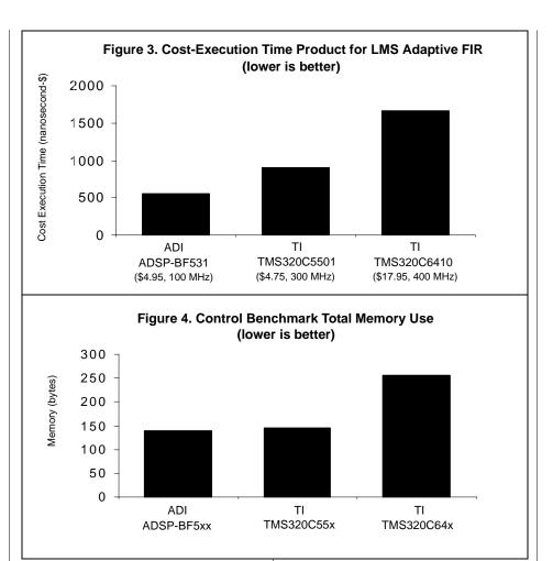
Control-oriented tasks usually constitute the bulk of an application's program memory requirements, but only a fraction of the application processing time. Thus, in control-oriented tasks, minimizing memory use is usually a more serious concern than maximizing execution speed.
