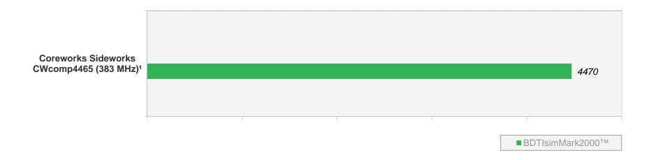
All processors benchmarked with 16-bit fixed-point data. All cores include at least 16 KB on-core memory and use worst-case clock speeds for theTSMC CLN65GP process and the Artisan Advantage core cell library. Vendors can choose different speed/area/power trade-offs; to understand the trade-offs, please view all BDTI metrics for each core. BDTIsimMark2000<sup>™</sup> scores may be based on projected clock speeds. For information, see www.BDTI.com/Services/Benchmarks.
